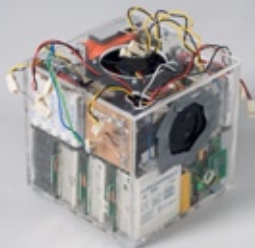
The inner cube carries most of the necessary parts like wireless connection, sensors and batteries
